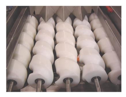
THE LAYTON/WELLIVER POCKET GRADER ALLOWS FOR GRADING TWO DIMEN-SIONS AT THE SAME TIME AND FEATURES A UNIQUE POCKET DESIGN FOR HIGH ACCURACY. THE GRADING ROLLS ARE CNC MACHINED FROM FOOD GRADE UHMW FOR EASY MAINTENANCE AND CLEANING. CAPACITIES ARE UP TO 4,000 POUNDS PER HOUR PER
